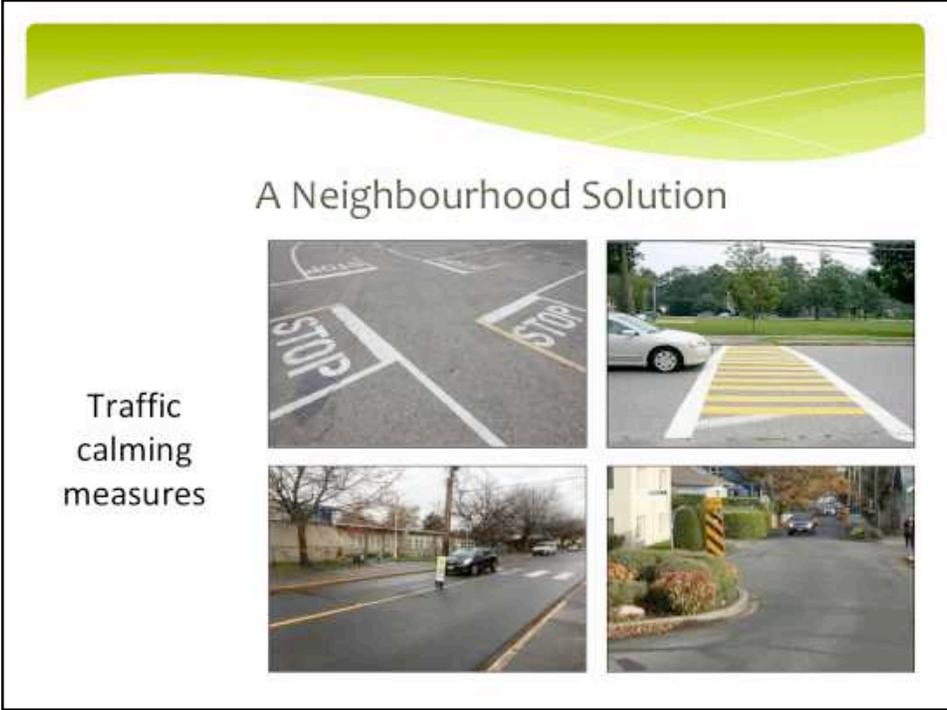
In addition to slower speed limits, additional traffic calming measures may be required in specific areas in the neighbourhood to aid compliance with these speeds. Furthermore, stop signs and crosswalks should be implemented based on pedestrian requirements rather than the standard regulations based on traffic counts.
