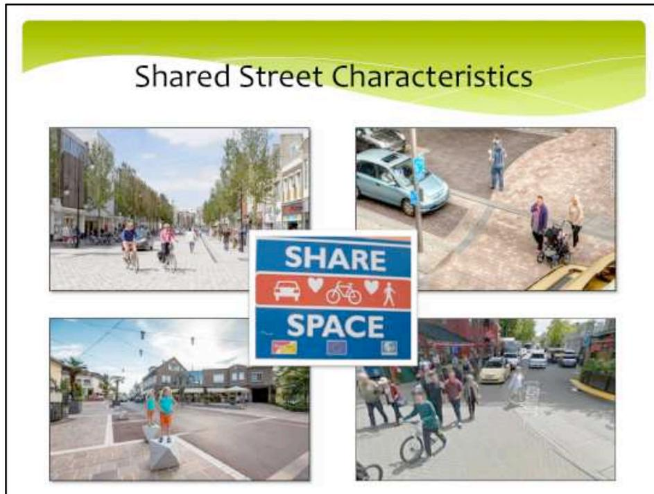
A shared street is a way of accommodating everyone by removing barriers between them. It minimizes the segregation of pedestrians and vehicles, by using materials and design that reflect different uses and allows for ebbs and flows between different modes of transportation. In shared street all modes of travel are considered equal.
